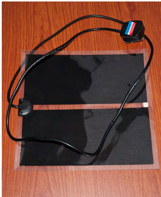
Fig. 5. The heat pad was supplied with zero instructions and no markings indicating rating.
