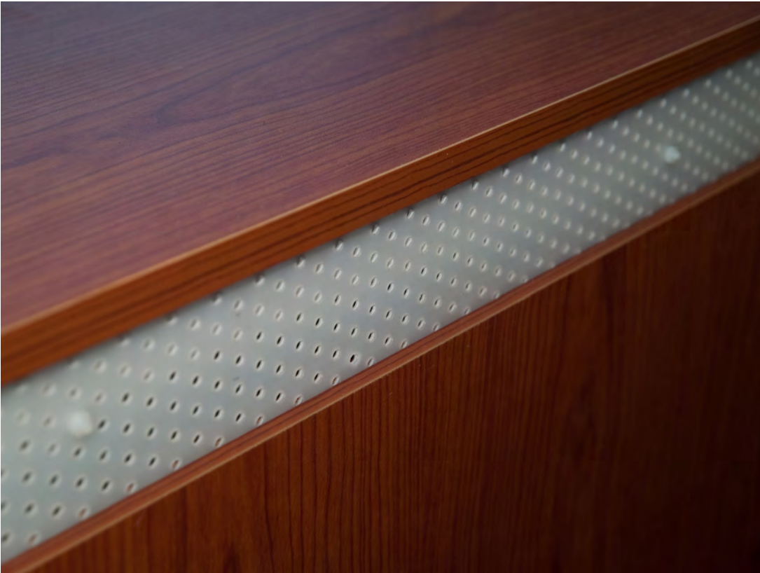
Fig. 12 The small ventilation grille at the rear was completely inadequate to permit effective convection cooling within the vivarium. This contributed to the severe overheating problems recorded in these tests.
